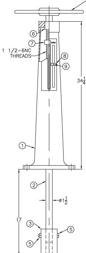
The F-5505-T indicating floor stand is for non-rising stem valves where open/close valve indication is needed. Floor stands are of high strength cast iron and may be provided with extension stems of steel, stainless steel or bronze as specified.
