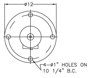
NOTES: POINTER TRAVELS 1" WITH TURNS OF HANDWHEEL
