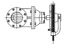
Chain Wheels are normally used for operation of valves located overhead. They are provided with chain guides to prevent the chain from slipping off the wheel. Chains can be furnished rust proof if specified. chain Wheels are mounted directly on the handwheel, and are of approximately the same diameter.
